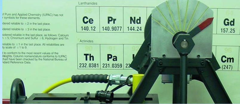
UTEC provides the ABL Friction Apparatus for clients who require in-house testing to determine the energy required to initiate a sample by friction energy application. The primary parts of the test apparatus are a moving anvil upon which the test sample is placed, a stationary wheel that applies a load to the sample, and a swinging pendulum that strikes the anvil to move it under the stationary wheel.
